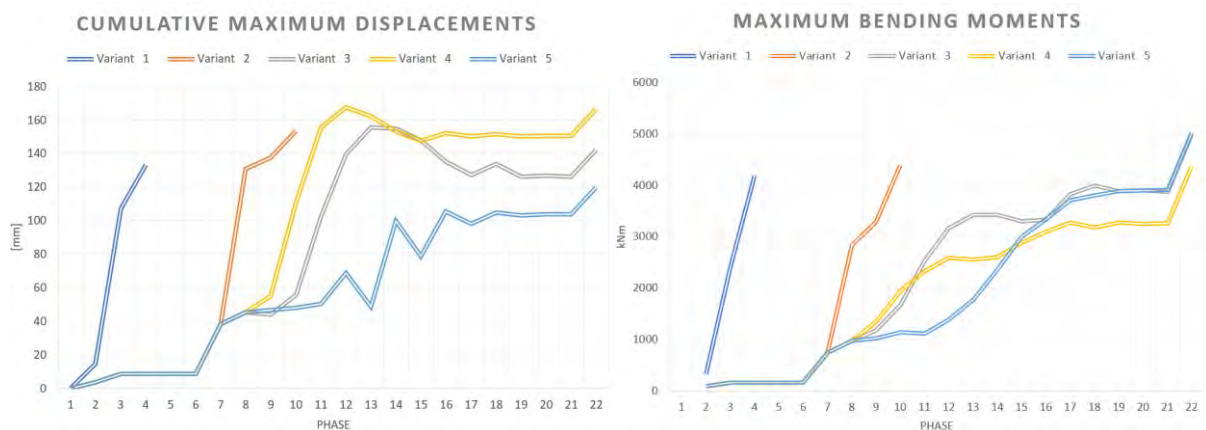
Figure 2. Results summarized in cumulative displacements and bending moments by phases
