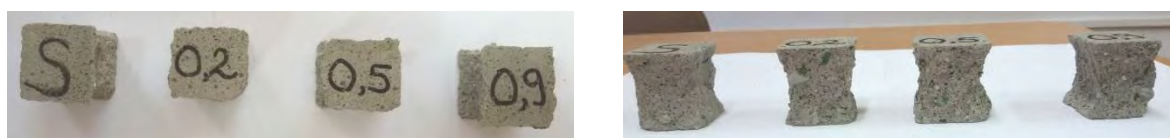
Figure 3: Standard mortar and mortars with glass wastes after tested at 28 days at compressive strength
