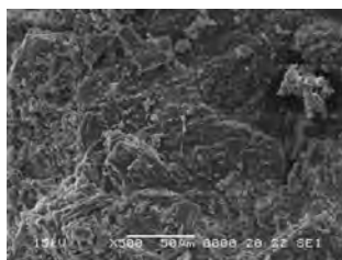
Figure 3: Structure of CSIV 20P plaster mortar at 500x resolution (Siomin, 2022)
