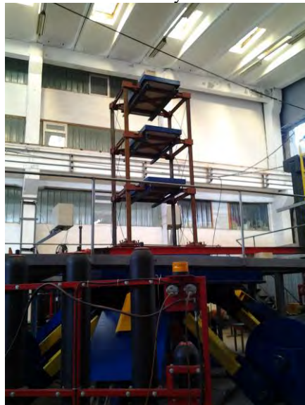
Figure 1: The Experimental Model on the Shaking Table
